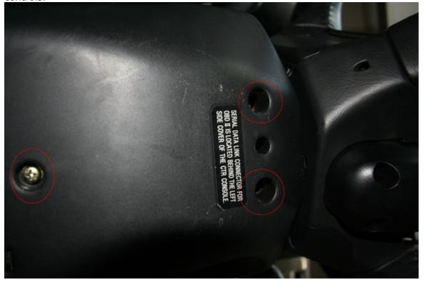
3. Unbolt the 2 circled 12mm nuts. The steering wheel should drop now and clear the dash bezel. (torque to 12 lb-ft when reinstalling)
