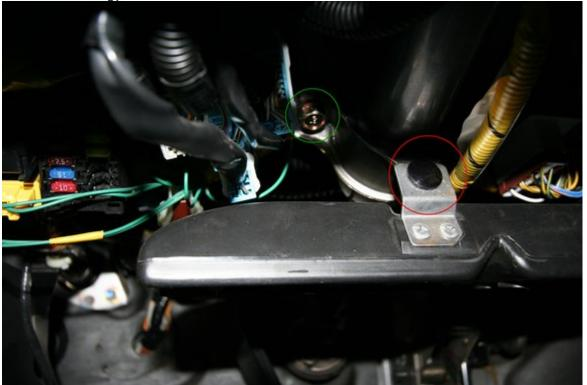
2. Unscrew the 3 screws circled. Then carefully remove the lower half if the shell around the wiper/light controls.
