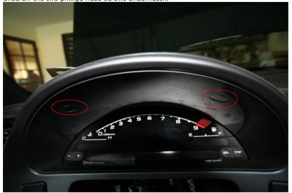
5. Using a flathead wrapped in electrical tape, carefully pry the dash bezel off without damaging the plastic. (The area below the defrost and cruise control button are nice places to stick your screwdriver in since you can't see if you bent the plastic.) After you've freed the bezel from its clips, be sure to unclip the electrical connectors. There is one for the Engine start button, radio controls, cruise control, defrost, and a/c controls.
