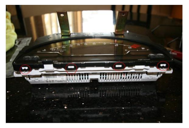
10. This is what it should look like with the black trim off. Make sure the surface of the gauge cluster is free of oil and dust before applying the CF trim.
