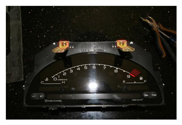
8. Using a mechanics pick or small flat head, unclip these circled clips. There is one on each side.
