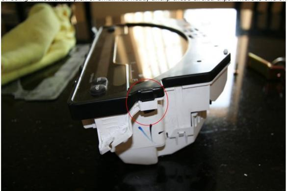
9. Carefully unclip the circled clips with a mechanics pick/flathead(be very careful not to crack these). The black trim should now come straight off.
